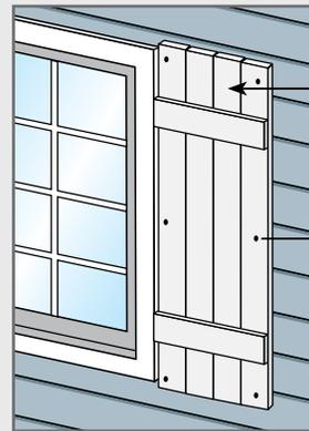
MiraTEC trim can be used to make decorative shutters. The shutter must be fastened to the home a minimum of 24" on center around the perimeter of the shutter as shown in the illustration. Working shutters are not covered by the MiraTEC limited warranty based on the inability of providing adequate fastening on the non-hinge side of the shutter.
