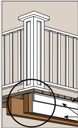
When facing the skirt boards on deck, properly flash the top edge to prevent water from getting behind the trim.
