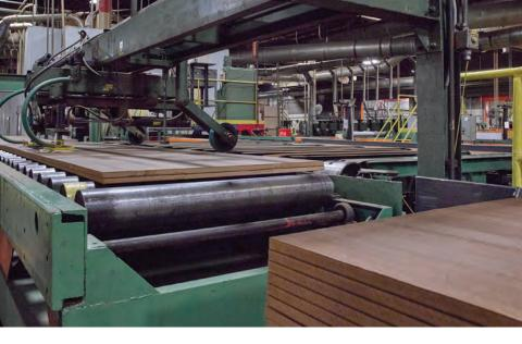
Next, the rough edges are cut from the mat. At this point, the trim is manually inspected at the grading station by carefully trained operators. Due to the precision of the TEC™ process, the yield rate is nearly 100 percent. JELD-WEN is committed to delivering a high quality product – boards are tested
