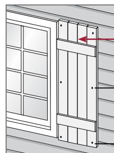
MiraTEC trim can be used to make decorative shutters. The shutter must be fastened to the home a minimum of 24" on center around the perimeter of the shutter as shown in the illustration. Working shutters will not be covered by the MiraTEC limited warranty based on the inability of providing adequate fastening on the non-hinge side of the shutter.
